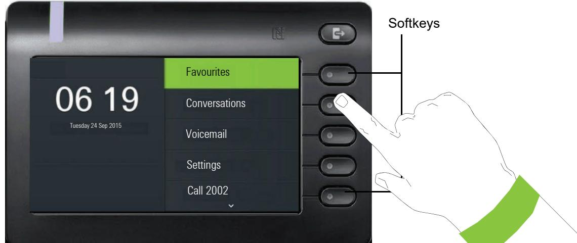
Some FPKs on the main menu display a status using LED colour and cadence. As you scroll through the menu, the LED on the corresponding key updates to reflect the state of the currently highlighted item.
