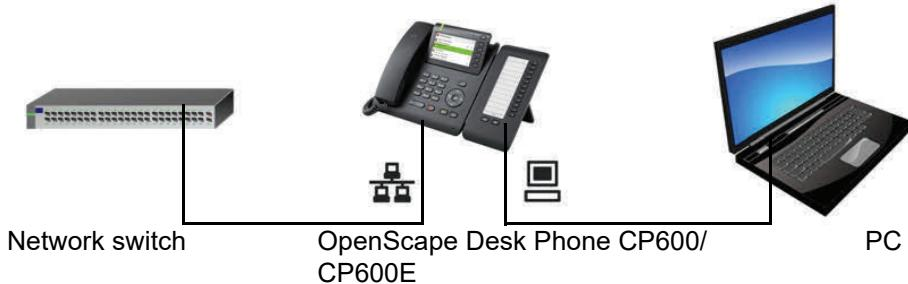
Using this connection option saves a network port for the switch used and allows shorter network cables to be used.
