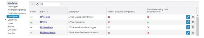
A running event plan is terminated and restarted if the same event is sent from the same endpoint. This can prevent the execution of further phases. With SIP-DECT 10.0 the option is introduced that a running event plan continues to run and further events of the same type from the same endpoint are ignored until the running plan is terminated.
