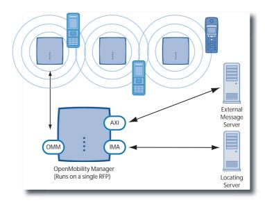
The OpenMobility Manager (OMM) and the OM Integrated Messaging & Alerting service (OM IMA) both run on a single DECT base station or on a dedicated Linux server system. The OM Locating application uses the IMA service to send messages to DECT phones. Other external messaging solutions, such as a message server or an alarm server,
