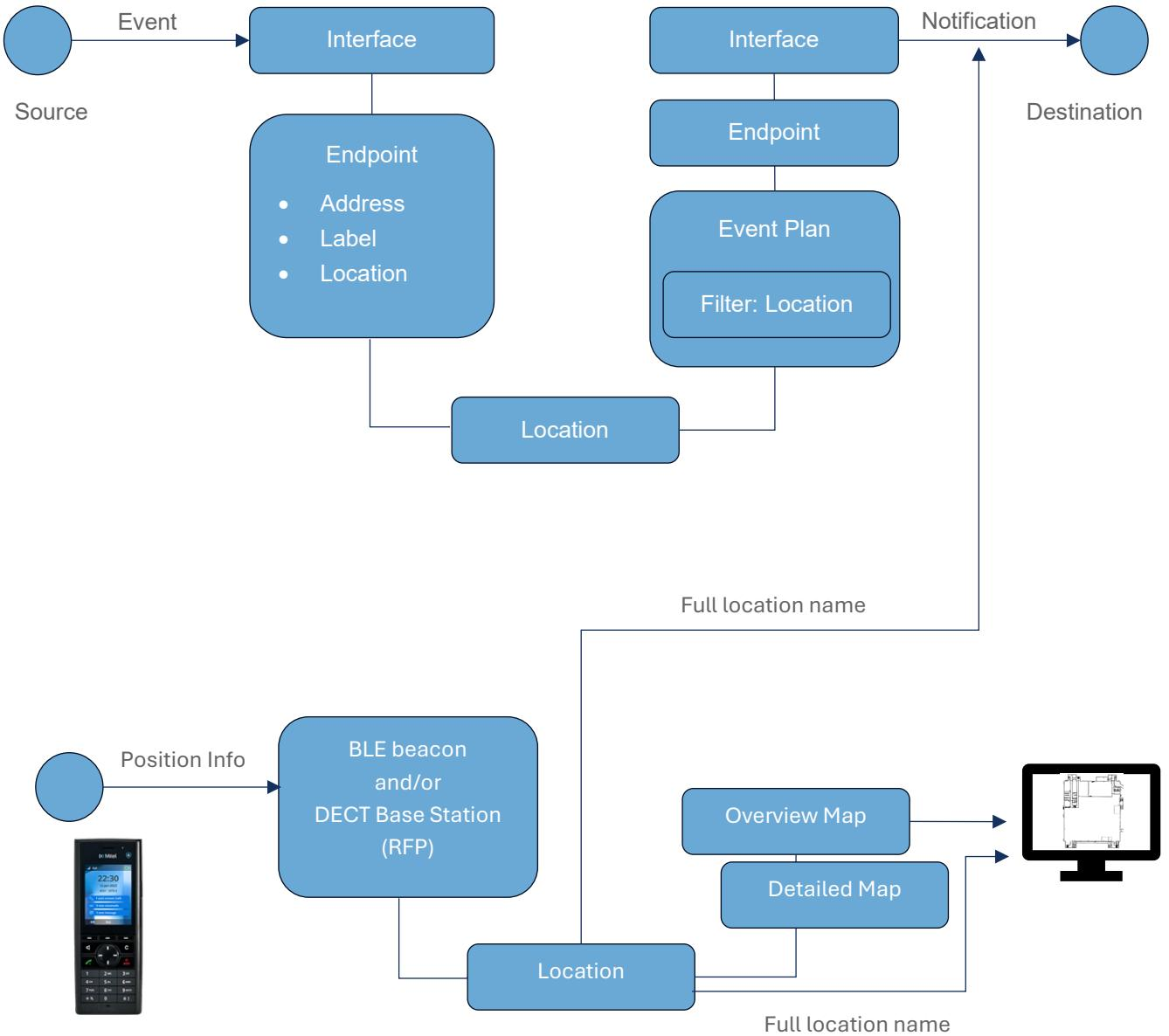
A Linux Server installation of the Event Manager is required to support DECT and/or BLE locating.
