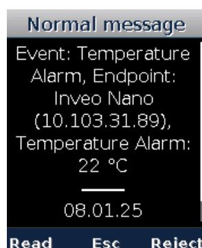
15. In case this did not happen, you may enter the SNMP interface's "Simulator/Trace" tab, tick the boxes "Data received" and "Additional Info" under "Trace" and start the trace. Once an SNMP notification has been received, a message will be displayed after the received notification, telling you what ended up happening while processing the
