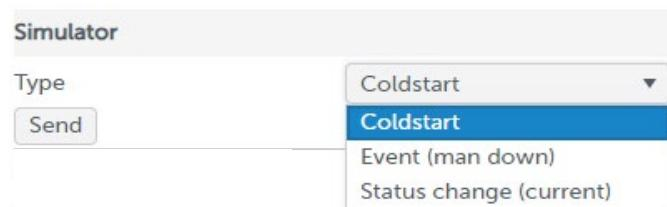
In order to see what the Event Manager sends, start the trace and check "Data sent". This is useful to test if this SNMP interface is correctly configured for sending traps as well as to check if the trap receiver outside the Event Manager handles traps correctly. Data sent by the Simulator is in the correct format, but data itself may or may not be correct.
