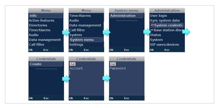
8 Perform a user login at the DECT phone to authenticate the user with the provider services. Open the System menu (press and hold the menu softkey ) and select Administration -> User login:
