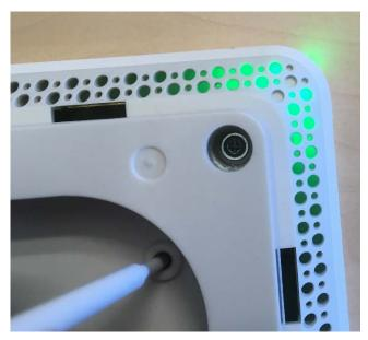
**9** Keep the button pressed until it starts flashing blue (approximately 5 seconds).
