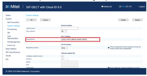
17 The RFP automatically restarts after applying a valid Cloud-ID Key.
