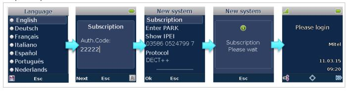
21 The following workflow is based on a scenario where provisioning is used. If the provisioning server requires system credentials, you must enter them to authenticate the SIP-DECT with Cloud-ID (SDC) system at the provider services.
