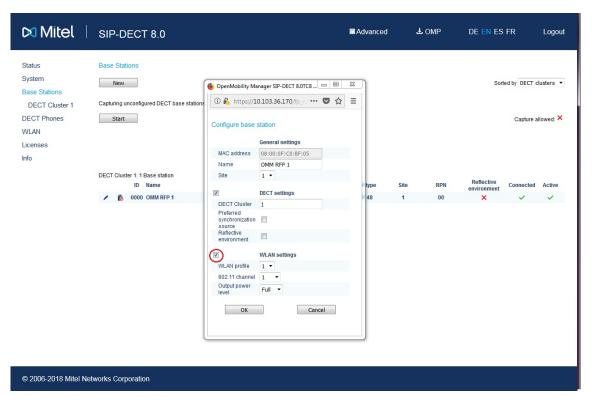
The selected WLAN channels have a default bandwidth of 20 MHz. If the WLAN profile options like HT80/ HT40 MHz is activated, the necessary center channel is automatically selected in the corresponding areas during the configuration itself.
