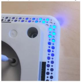
**10** Release the button while the LED is flashing blue to switch to SDC mode.
