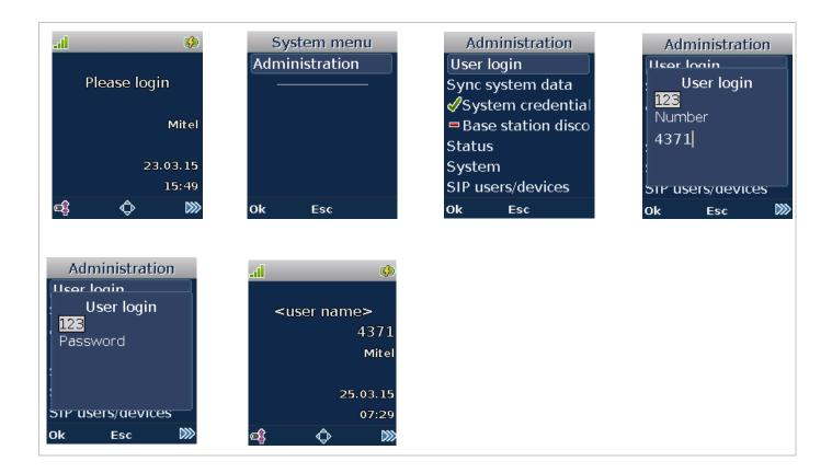
The DECT phone's standard screen displays the user's name as well as the phone number that is configured with the SIP user account. The DECT phone is ready to be used for telephony functions.
