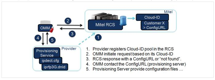
The OMM (re)loads all external configuration files on startup and when explicitly triggered.
