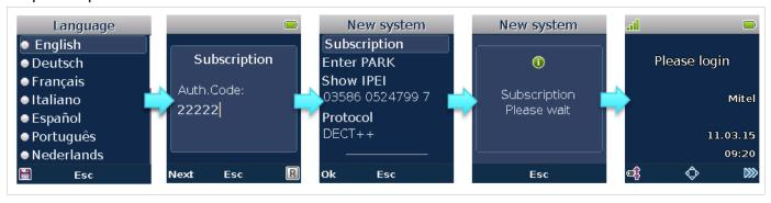
You can log in to the DECT phone using either of the following methods:
