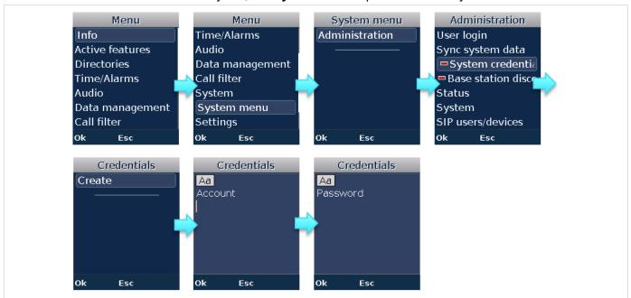
23 Perform a user login at the DECT phone to authenticate the user with the provider services. Open the System menu (press and hold the menu softkey ) and select Administration -> User login:
