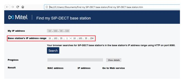
i) Check and adjust the Base srations' IP address range if necessary.
