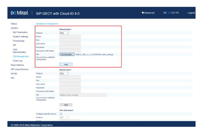
**Note**: Activate the option **Preserve user device relation at DB restore** in the new OMM. The new OMM restores the relation between the user and the DECT phone during DB import. If this option is not set, then all dynamic users get logged out from their DECT phones when importing the OMM DB into the new OMM.
