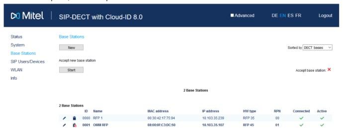
After the automatic SW update, the SW version mismatch disappears, and the RFP is automatically put into operation. The name of the previous OMM RFP can be changed to avoid confusion.
