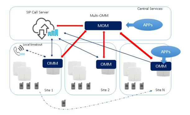
The MOM maintains a connection to each OMM in the system and manages all user and device operations, including roaming between sites. In addition, the MOM provides messaging and alerting support across all sites in the system, and provides an interface through which applications attached to the OMMs at different sites can communicate.
