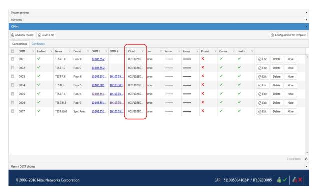
Optionally, you can click on the IP address of the OMM record (**OMM 1** or **OMM 2** field) to open the OMM web interface in a new browser window.
