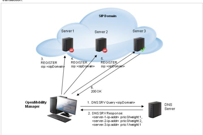
To prevent situations where the OMM tries to contact servers that are unreachable (out of service) with each new transaction, the OMM offers a blacklist feature. If there is no answer from a SIP Call Manager, this specific server can be put on a blacklist and is not contacted anymore for a configurable time ("Blacklist time out") for all subsequent SIP transactions.
