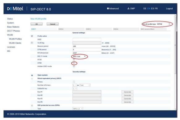
HT80 includes the HT40/HT20 bandwidth setting. A channel with a bandwidth of 80 MHz occupies 4 WLAN channels with a bandwidth of 20 MHz.
