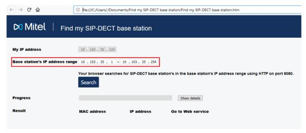
i) Check and adjust the Base srations' IP address range if necessary.
