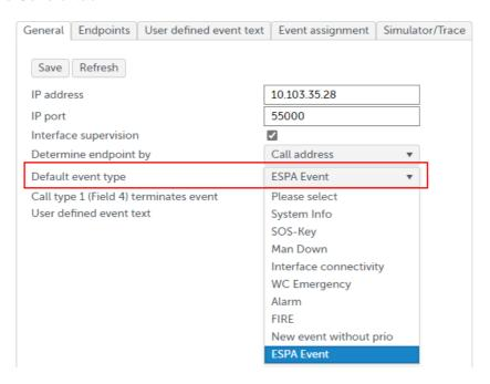
Rules can be defined in the **Event assignment** tab of the ESPA interface configuration, as shown below.
