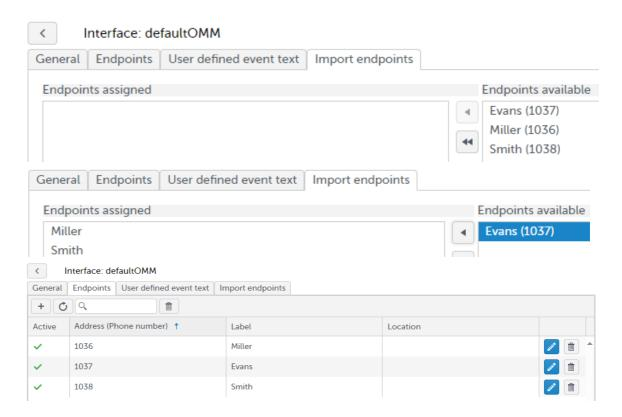
7. Assign the endpoints to the default location root as shown below.
