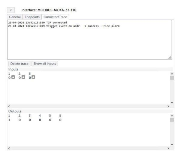
In the Outputs part of the **Simulator/Trace** tab the activity on output port 1 (in this example there is a light connected) is visible and in the trace part of the tab the handled trigger event at the incoming port 1 (triggered by the switch connected physically to this port or by pressing the button 1 in the Inputs part) is documented.
