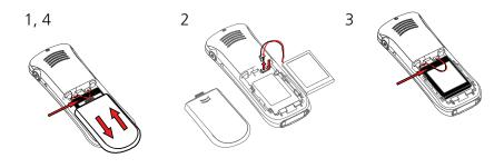
Figure 11: Easy Replaceable Battery.
