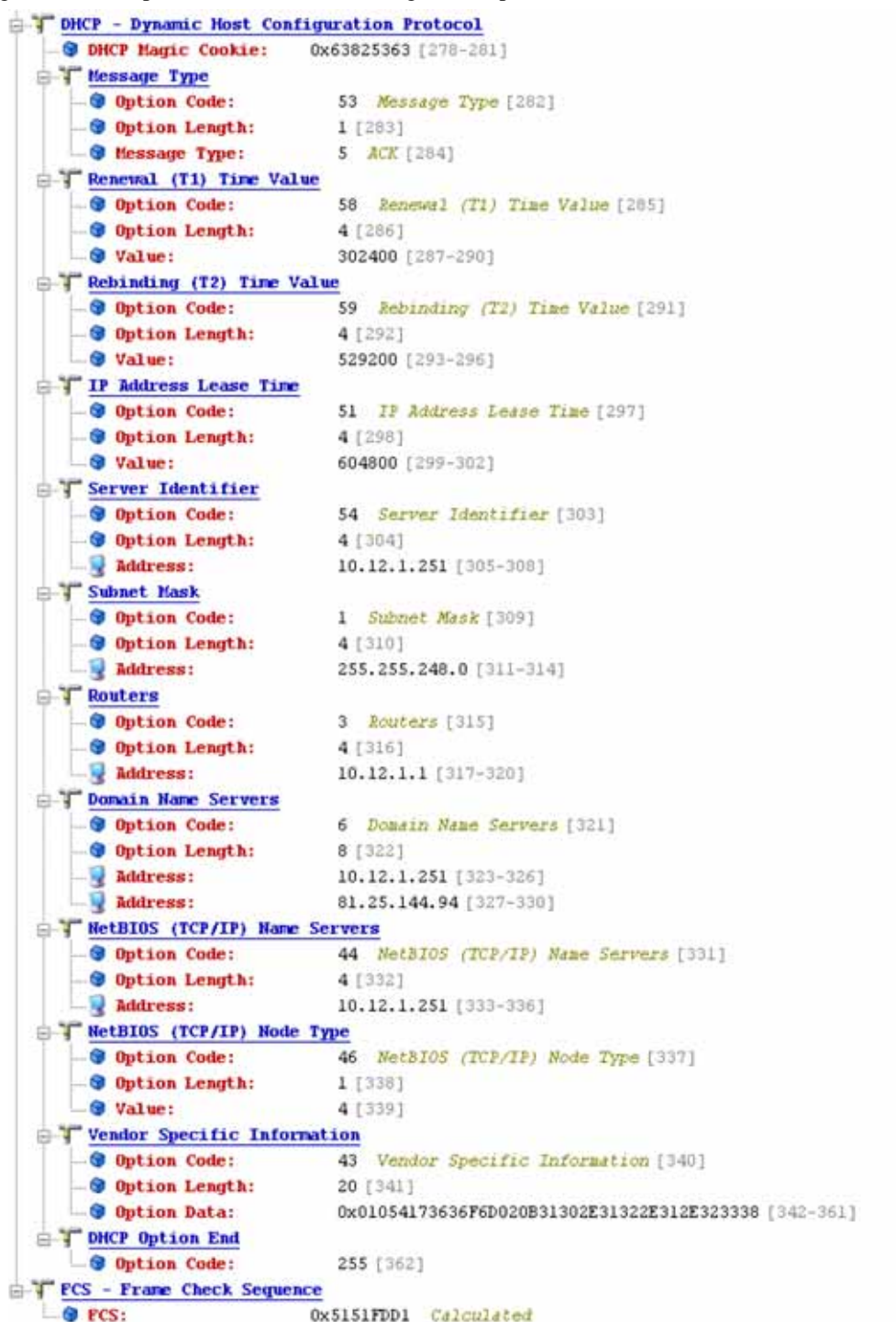
Figure 23. Example of a DHCP Acknowledge (Omnipeek trace).
