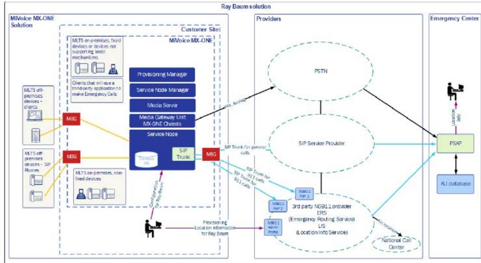
The following figure shows a high-level view of the MX-ONE RAY BAUM architecture for a networked MX-ONE system that uses SIP tie-line.
