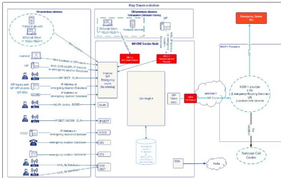
The RAY BAUM solution comprises of three main components: devices, MX-ONE, and the NG911 provider.
