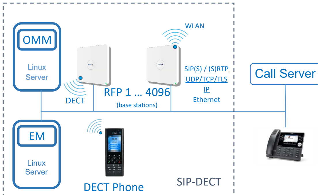
Figure 2: SIP-DECT Architecture Overview - OMM and EM running on Linux Server
