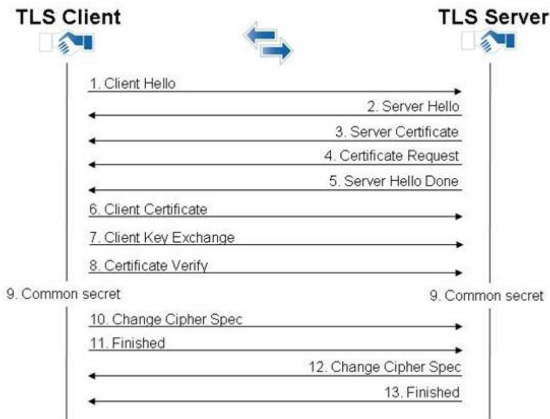
Figure: 2: Mutual TLS handshake. The server also requests the client's certificate. The client and server both authenticate the other's identity.
