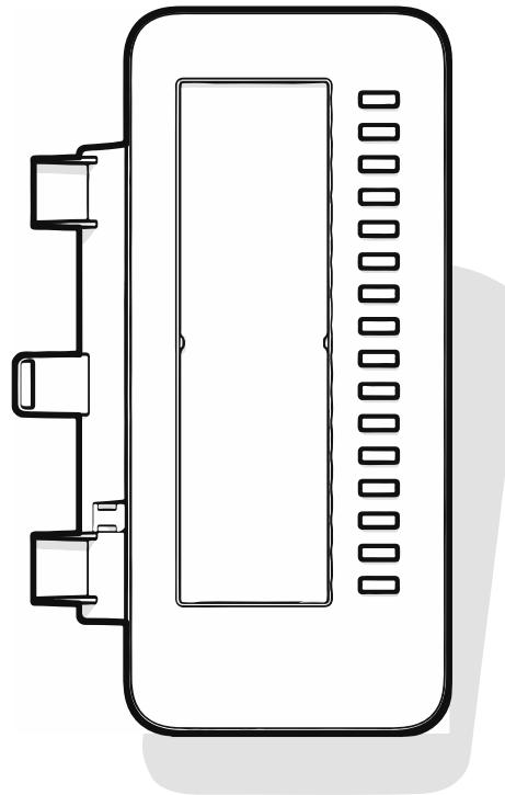
The KM410 is an optional key module attached and connected to the right side of the phone that provides an additional 16 illuminated and programmable function keys (see "Programmable function keys" → page 64).
